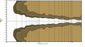
Dispersion angle diagram of a single X15 HiQ in vertical (top) and horizontal (bottom) plane using lines of equal sound pressure at -3db, -6dB, -12 dB.
