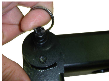
(2) Release pivoting arm locking pin
