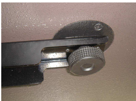
(7) Rotate the SBI5P to the desired angle and secure using the tilt adjustment knob (pivoting arm locking pin automatically secures the U-bracket as the adjustment knob is tightened)
