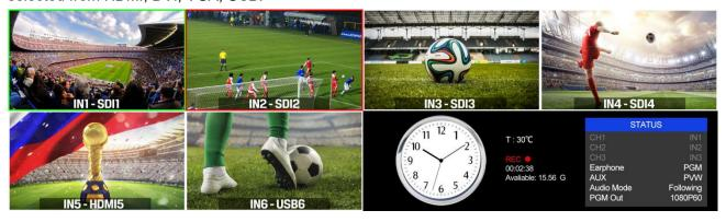
3) The lower right corner displays the menu and status information. The CH1, CH2, CH3 are the channel selection of the 3 audio sources for audio mixer. There is a real-time Digital clock/ Analog clock displayed beside the menu.
