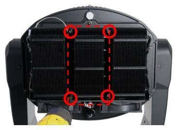
5. Remove (4x) 3mm hex-head screws holding the center heatsink module.
