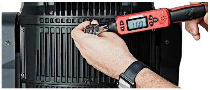
The (12x) hex-head screws holding the panels MUST be tightened with a torque wrench
