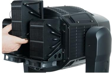
6. Unclip the center heatsink module safety cable.
