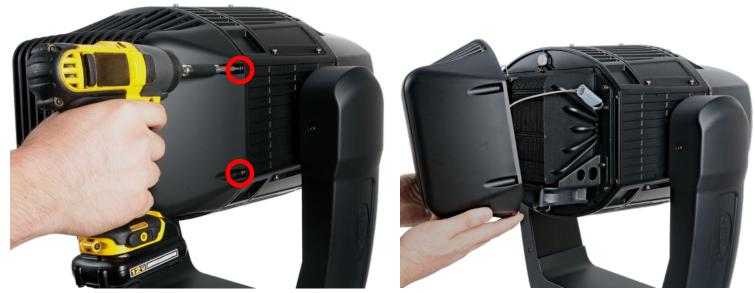
3. Remove (4x) 3mm hex-head screws to remove rear cover.
