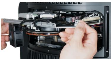
9. Carefully remove the effect module from fixture.
