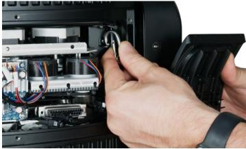
4. Unclip the panel safety cable one side of the head.
