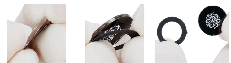
14. Carefully remove the retaining ring washer attached to the GOBO. SAVE RETAINING RING WASHER FOR USE WITH THE NEW REPLACEMENT GOBO! **RETAINING RING MUST BE USED IN ORDER TO PREVENT GOBO BURNING!**
