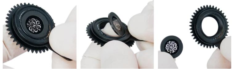
13. Carefully separate the GOBO disc from the GOBO Holder.
