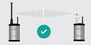
Always mount the devices so the device antennas are at the same height.
