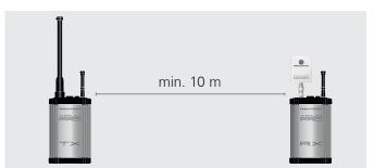
For a setup with a single transmitter and a number of receivers the minimum distance between the TX and any RX should be 10 meter.
