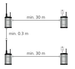
If several transmitters are used in the network, observe the following: Select the transmission channel for the TX in the app so at least one
