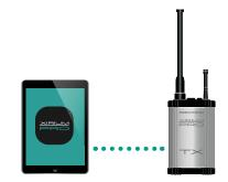
**Stand-alone mode** Only 1 device is directly connected to the app.
