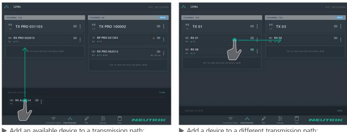
Add an available device to a transmission path: Under Available Devices, use drag&drop to add the device to the transmission path. Add a device to a different transmission path: Tap the device and drag it to the desired transmission path.
