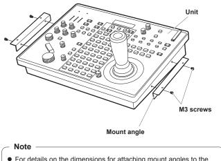
• For details on the dimensions for attaching mount angles to the unit, refer to "Appearance" (page 11).
