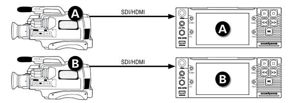
In this scenario, each camera is its own master video sync source, but the PIX 270i is the source of the timecode. The PIX 270i records its files based on the camera's clock. The heads will match perfectly, but the tails may drift depending on the cameras' clocks.
