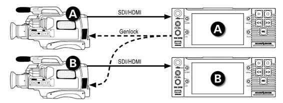
In this scenario, a PIX 270i is the master sync source for multiple cameras, each with or without their own PIX acting as a recorder. Because of this locked connection, the cameras can be run indefinitely and be assured of frame-accurate sync with no possibility of drift.
