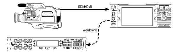
The wordclock output on the PIX 270i is synchronous with incoming video signal. The wordclock output can be used to sync external audio recorders to any camera. To enable wordclock output, set Setup Menu item [Timecode/Sync - Sync Out] to Wordclock, Follows Video In.
